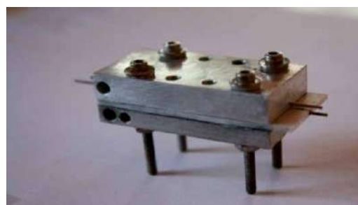
Figure Flow electrolyzer for the co-electrolysis of CO 2 to CO or ethylene on the cathode, and glycerol to lactate and/or formate on the anode
