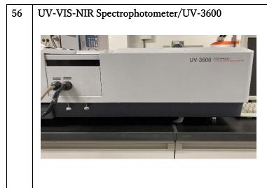
The UV-3600 can handle measurement with highly precise transmittance and reflectance, and uses three detectors to handle a range going from the ultraviolet region to the near-infrared region. Using a high-performance double monochromator makes it possible to attain an ultra-low stray-light level with a high resolution.
