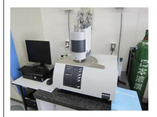
Thermal stability, decomposition behavior, composition, phase transitions, melting processes to be analyzed with this instrument comprehensively and quickly.
