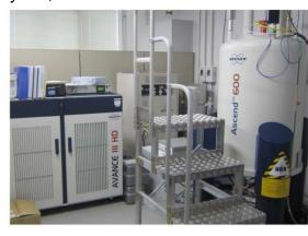
NMR is a way to detect spin states of a target nucleus contained in a material. This technique is possible to predict the type and structure of the elements present in the unknown materials. This 600 MHz Bruker ultra shielded magnet equipped with a 5 mm liquid probe and 3.2 mm CP MAS probe can access the wide range of experiments to determine the elements and structures. Bruker Icon NMR also facilitates all of the measurement processes, which can broaden the users of this equipment.
