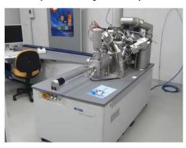
Time-of-Flight secondary ion mass spectrometry (TOF-SIMS) is a very sensitive surface analytical technique, well established for many industrial and research applications. It provides detailed elemental and molecular information about the surface, thin layers, interfaces of the sample, and gives a full three-dimensional analysis. The use is widespread, including semiconductors, polymers, paint, coatings, glass, paper, metals, ceramics, biomaterials, pharmaceuticals and organic tissue.
