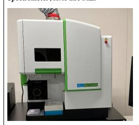
This is an elemental analysis system using inductively coupled plasma (ICP) as a light source.
