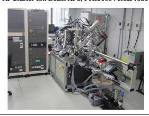
XPS (X-ray Photoelectron Spectroscopy) is for the elemental analysis of a specimen and can measure elemental compositions, chemical and electronic state quantitatively. In this equipment, Ar cluster ion beam system is attached to etch the sample surface mildly for intentionally exposure of deeper layers of the sample in depth-profiling XPS.
