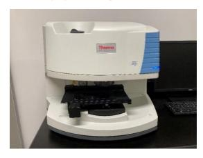
Fourier Transform Infrared Spectroscopy with 2D mapping capability to characterize the chemical composition and microscopic structure of polymer composite surfaces. It can be used to analysis the surface reaction products and deposited materials arise from sliding between polymer and metals.
