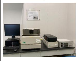
The hall effect measurement system is suited for evaluation of electronic conductors semiconductors. It enables measurement of resistivity, carrier concentration and mobility on a wide range of semiconductors and with minimum effort in sample preparation. It is designated as a modular system and the basis instrument can measure sheet resistivity up to a few Mohm/square and Hall voltage of a few  $\mu$  V.
