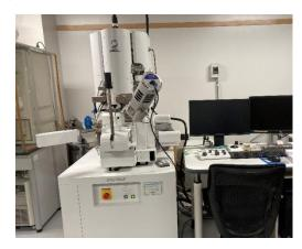
JSM-7900F Field Emission Scanning Electron Microscope is equipped with a new electron optics control mechanism that can take full advantage of the characteristics of a strongly excited conical objective lens (Super Hybrid Lens), which is a hybrid of an In-Lens Schottky field emission (T-FE) electron gun and an electrostatic lens. You can easily observe the sample surface with ultra-high resolution and perform various analyzes, such as EDS, WDS, EBSD, and CLD.
