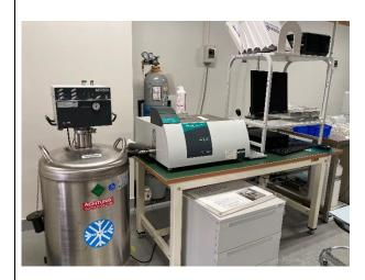
Differential scanning calorimetry, DSC, is the most-employed thermal analysis method for soft matter. DSC allows to measure the amount of energy absorbed or released by a sample when it is heated or cooled, providing quantitative and qualitative data, such as melting temperature, heat of fusion, glass transition temperature, crystalline phase transition temperature and energy.
