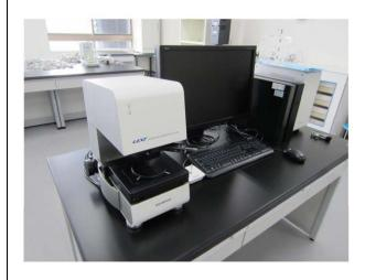
The machine is designed for nanometer level height imaging and roughness measurement.
