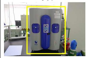
The Inverse Gas Chromatography-Surface Energy Analyzer (iGC-SEA) measures the surface energy of a sample by subjecting the sample to vapor probes of known properties and investigating the interface between the surface of the sample and other molecules. The vapor's retention time is measured by a Flame Ionization Detector (FID). Varying the vapor probe molecule, flow rate, temperature, or column conditions elucidates a surface and bulk properties of the sample.
