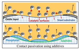
With the continuous increase in bearing steel strength, a new type of failure was observed in rolling elements related to the presence of atomic hydrogen in the material. High strength steels are particularly susceptible to hydrogen embrittlement
