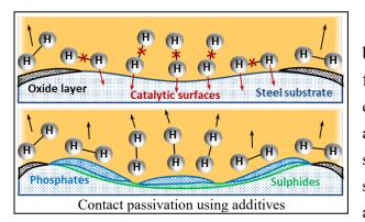
With the continuous increase in bearing steel strength, a new type of failure was observed in rolling elements related to the presence of atomic hydrogen in the material. High strength steels are particularly susceptible to hydrogen embrittlement and can experience premature failure
