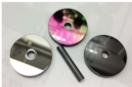
Figure 2. Disc and pin specimens
