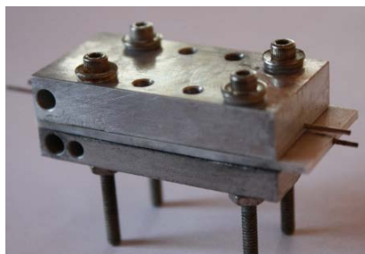
Figure 1. Picture of the electrochemical flow reactor for the electrochemical reduction of CO 2 .
