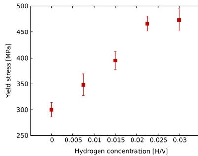
**Figure 4.** Flow stress of the deformed vanadium pillars at 5% strain for varying hydrogen concentrations.
