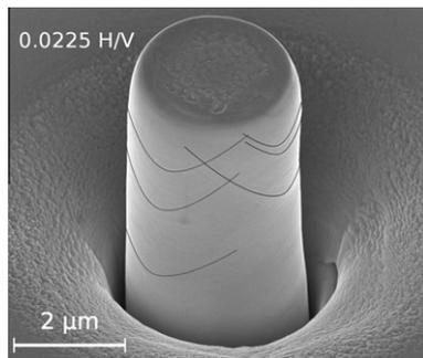
**Figure 2.** SEM micrographs of a deformed vanadium micropillar with a hydrogen concentration of 0.0225 H/V (same pillar as in Fig. 1, but rotated by an angle of  $180^\circ$ ). The side surface of the deformed pillar reveals many relatively small steps indicated by black lines. Furthermore the micrograph shows that all possible slip planes were used for the deformation, see also Fig. 1.
