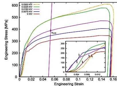
**Figure 3.** Stress–strain curves of the pillars of Fig. 1. Higher hydrogen concentration leads to higher flow stress. Furthermore, it can be seen that the serrations in the beginning of the curves (inlay, marked by arrows) disappear.
