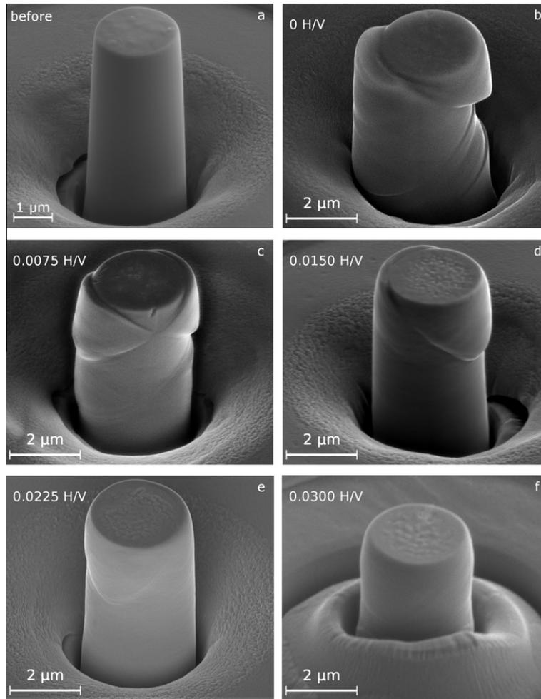
**Figure 1.** SEM micrographs of an as-prepared pillar (a) and deformed vanadium micropillars (b–f) showing different deformation morphologies: without hydrogen the pillar deforms on localized glide planes (b–d), increasing hydrogen concentration changes the deformation to a barrel-like shape (e and f). The images are taken at a tilt angle of  $45^\circ$  with respect to the sample surface.
