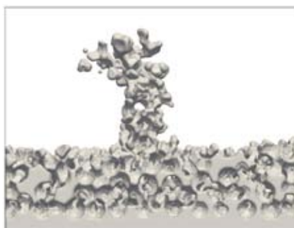
Fig. 2 The result of a CO 2 flow simulation based on LBM. Anisotropic CO 2 flow is simulated in the porous model with slit-like structure, which has different pore-size distributions between the slit and the other part.
