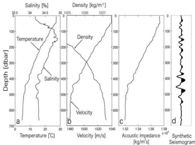
**Figure 3.** Vertical profiles of (a) temperature and salinity obtained from CTD data off the Ashizuri peninsula on 17 September 1994, (b) acoustic velocity and density calculated from temperature and salinity, (c) acoustic impedance calculated from acoustic velocity and density, and (d) synthetic seismogram calculated from acoustic impedance.
