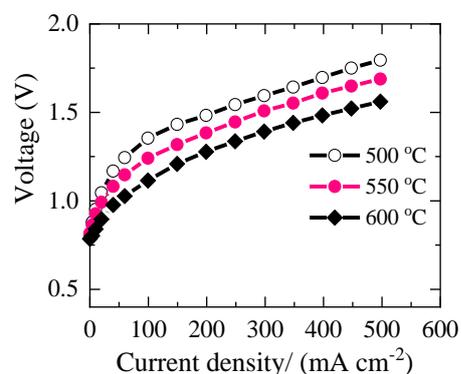
Fig.1. steam electrolysis I-V curve performance with ~20  $\mu\text{m}$  thick  $\text{BaZr}_{0.44}\text{Ce}_{0.36}\text{Y}_{0.2}\text{O}_{2.9}$  electrolyte
