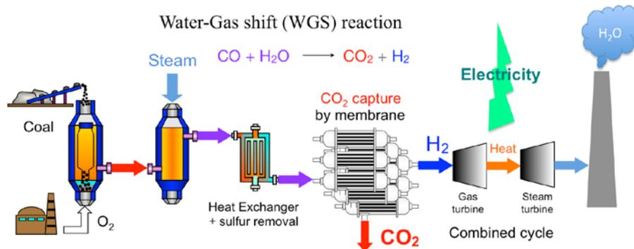
Fig. 1. Schematic drawing of CO<sub>2</sub> capture at an integrated gasification combined cycle (IGCC) plant
