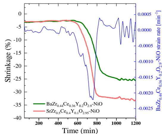
Fig. 1 Shrinkage of BaZr<sub>0.44</sub>Ce<sub>0.36</sub>Y<sub>0.2</sub>O<sub>2.9</sub>-NiO and SrZr<sub>0.5</sub>Ce<sub>0.4</sub>Y<sub>0.1</sub>O<sub>2.95</sub>-NiO cylinders prepared from the substrate single layers.
