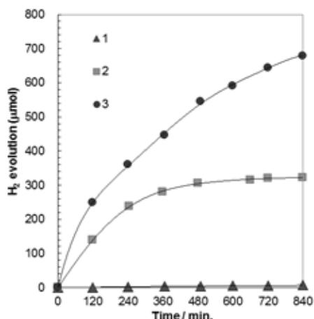
Fig. 2. Photocatalytic activities of the dyes **1–3** for water splitting reactions. Reaction conditions: 10 mL of 10 vol% TEOA aq., 33.0 mg dye–TiO<sub>2</sub>–Pt catalyst, pH = 7.0. A 300 W Xe lamp was used (the light below 420 nm was cut off by an optical filter).
